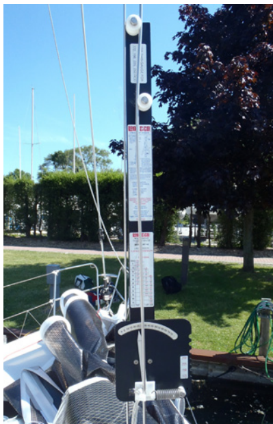
Measuring Rig Tension with the RT-10m Gauge
