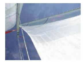
*Mark your spreaders:* Install 2 1" tape marks on your lower spreaders at 4" and 6" from the tip for future reference. We usually sail with the leech of the jib between these marks.
