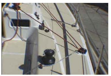
Trim to the cabin top so the trimmer does not have to move far off the rail to get to the winch and can see the sail and telltale. Keep the lazy sheet on the windward winch for inhauling. A good trimmer will mark his sheets to repeat trim settings without always
