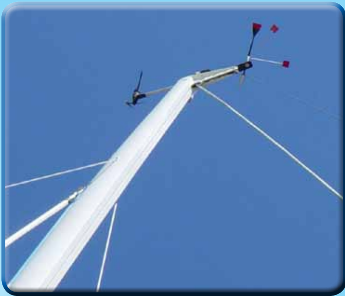
3. Masthead fly with calibrated arms for fast easy wind checks by skipper and crew.
