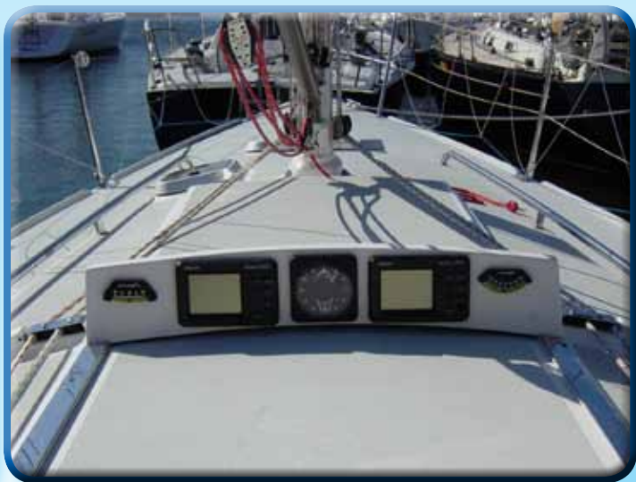
6. Instruments added at an easy location for the entire crew to see and use.
