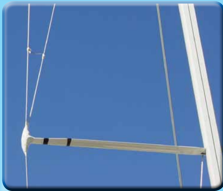
4. Reference marks for easy jib trim. Also note the lace lines on the V of the shrouds. This helps prevent the spinnaker from fowling in the V during a spinnaker takedown.
