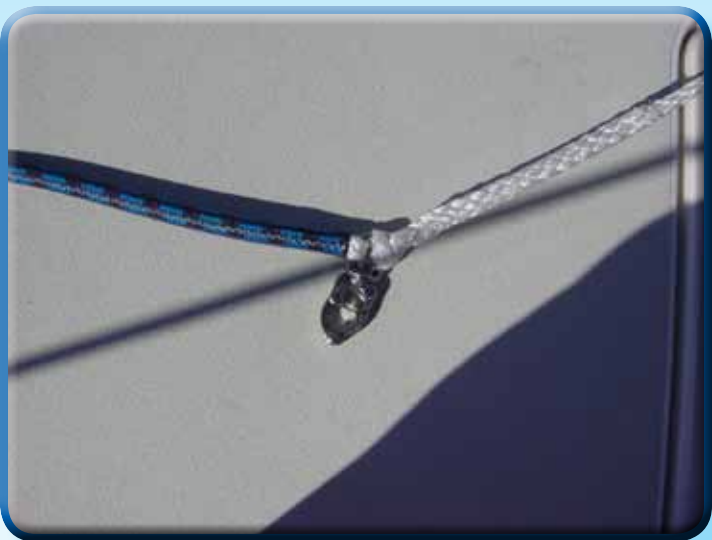
5. Tylaska shackle added to tack line and spinnaker sheets for fast easy spinnaker setup.
