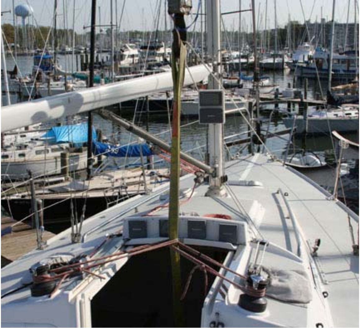
J105 Lifted By Single Point Lift
