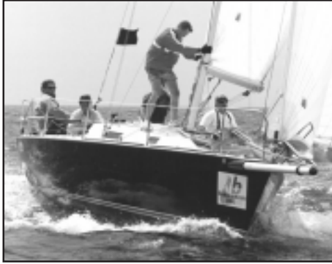
#4 POLE OUT: I use tackline to help the pitman get the pole all the way out; mastman stands to jump the set.
