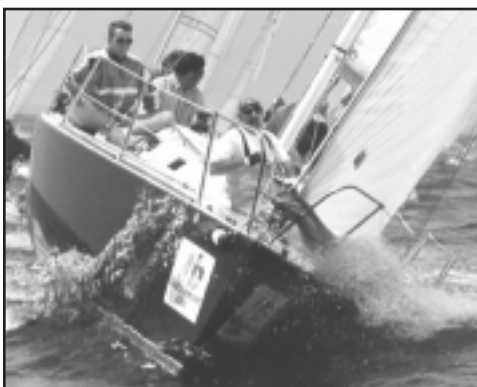
#2 TACK OUT: Hauling on the tackline to get the tack over the pulpit.
