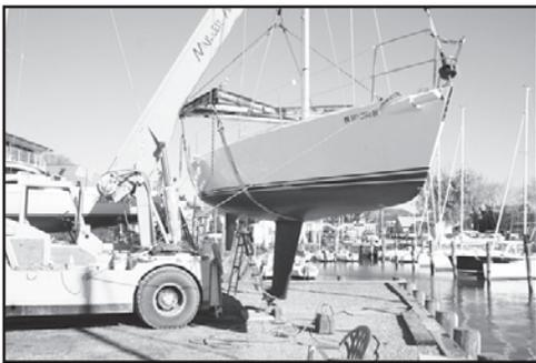
The lifting arrangement in action. The boom does not have to be removed, though it has been in this photo.
