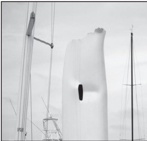
*This mast died of compression failure in Key West.*
